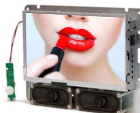
7" Open Frame displayer Available in standard & higher definition Available with trailing PIR & button modules
